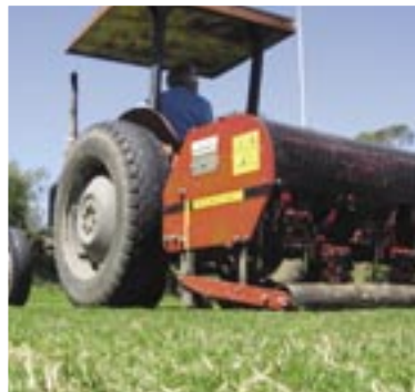
Sports field aeration -Vertidrain in action
